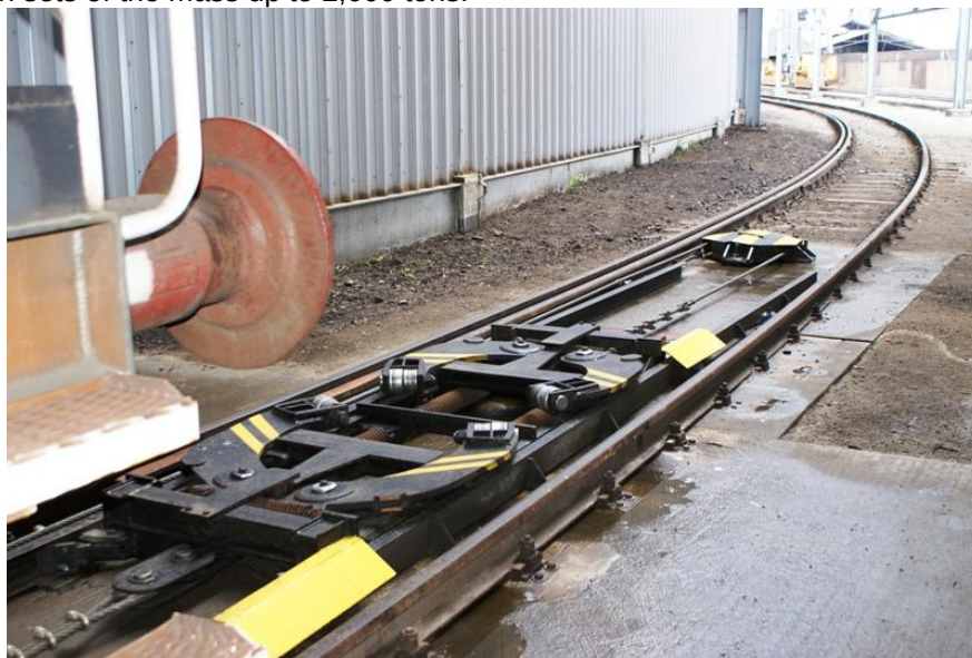
Fig. 2. A car puller mounted in the track (type UT-7, UNITOR)
